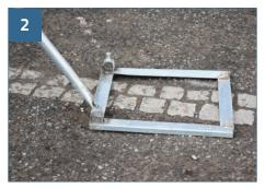
Connect the loading tray to other end of the support brace by removing the bolt and replacing through the hole in the support brace and tighten (recommended torque 15NM or 10lb/ft).
