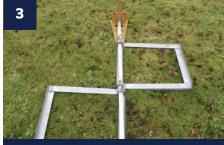
Slide 2x ZT loading trays onto the ZT bar as shown and tighten the 3 bolts closest to the base (recommended torque 15NM or 11lb/ft). Do not tighten the fourth bolt at this stage.
