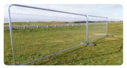
Insert the first and second fence panels into the first three blocks (centre holes) and connect with two couplers and tighten to 7NM or 5lb/ft. Repeat until installation is complete.
