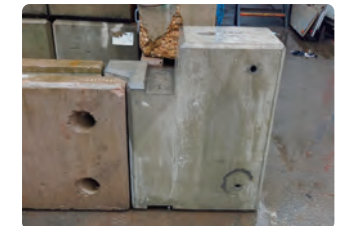
VCB End Section
